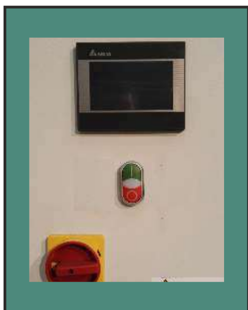
Frontal view of the control board of the TCS series, 230V - 50Hz or 400V - 50 Hz depending from the type of machine.
