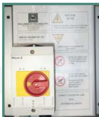
!"E" - magnetothermal switch with start and stop functions, with thermal protection of the motorvibrator;
